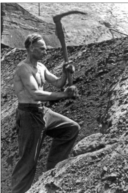
Lignite miner working with a single-point pick in an open cast mine, about 1956.
