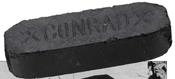
Lignite briquette for domestic use, compacted in the briquetting plant of the mine „Conrad” near Döbern, Size 18 cm x 5,5 cm
